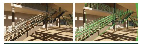
**Figure 26-5.** This image highlights the areas where a new diffuse ray is requested (green). Left: the camera is stationary. Due to the temporal antialiasing camera subpixel offset, the reprojection fails at geometry edges. Right: the camera is moving to the right. New rays are requested at geometric occlusions and areas that were not present in the previous view. Note the partially green walls due to a decrease in the density of accumulated samples.
