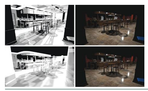
**Figure 13-11.** Hard shadows comparison. Visibility buffers (left) and rendered image (right) for the Pub scene with four lights, showing hard shadows rendered using our method (top) and shadow mapping (bottom).
