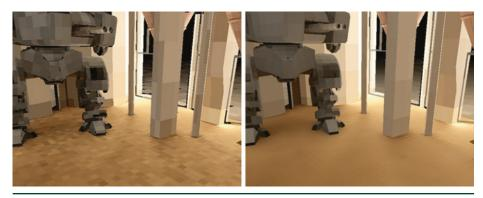
**Figure 23-10.** Left: light map data visualized after the merge and dilation operations. Right: light map data visualized after the denoiser step. In both pictures bilinear filtering is disabled to emphasize the noise reduction.
