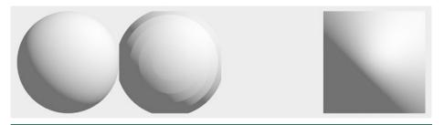
**Figure 7-3.** Four unit spheres (r = 1) placed at distances of (from left to right) 100, 2000, 4100, and 8000 from an orthographic camera. Directly implementing Equation 3 can result in severe floating-point precision artifacts, up to missing intersections altogether, as for the 4100 case.
