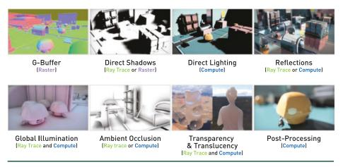
Figure 25-2. Hybrid rendering pipeline.
