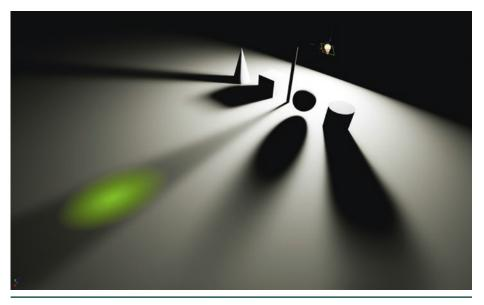
**Figure 19-5.** Visualization (in green) of a filter kernel used in our shadow denoiser. Notice how it is anisotropic and stretches along each penumbra's direction. (From Liu [7].)
