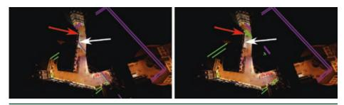
**Figure 18-7.** Visualization of the second level of the BVH when built using SAH (left) and SAOH (right); the AABB of the left child is colored in green whereas the one of the right child is in magenta. In both cases, 16 bins were used and all three axes were considered.
