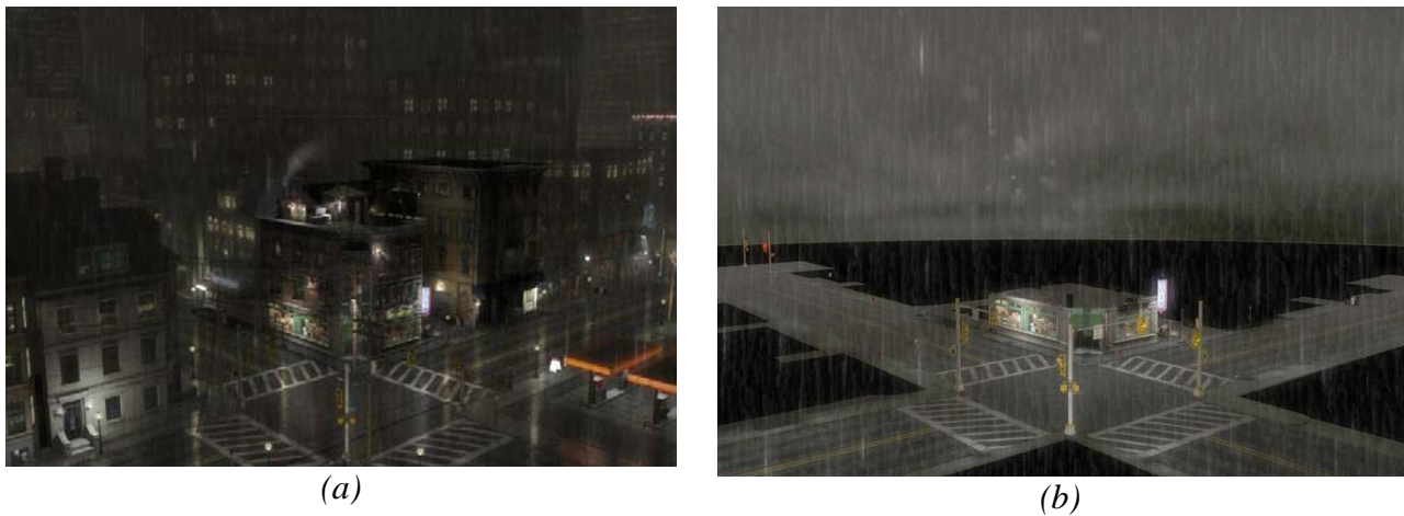
Figure 3. In (a) the entire scene is rendered with the use of 3Dc and DEC3N technology. Without using this technology, we are only able to fit a small portion of the original environment into the graphics card memory (b).
