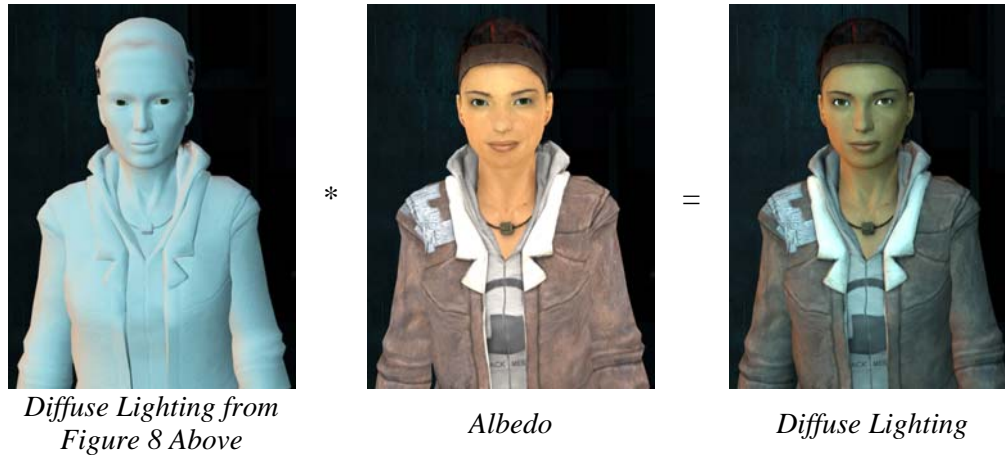
Figure 9. Diffuse character lit by two Half-Lambert terms and ambient cube
